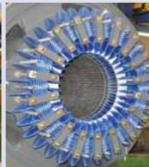
Special multi stage tooling was developed in-house to form and shape the unusual coil profile.
