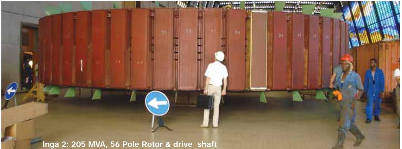
Inga 2: 205 MVA, 56 Pole Rotor & drive shaft
