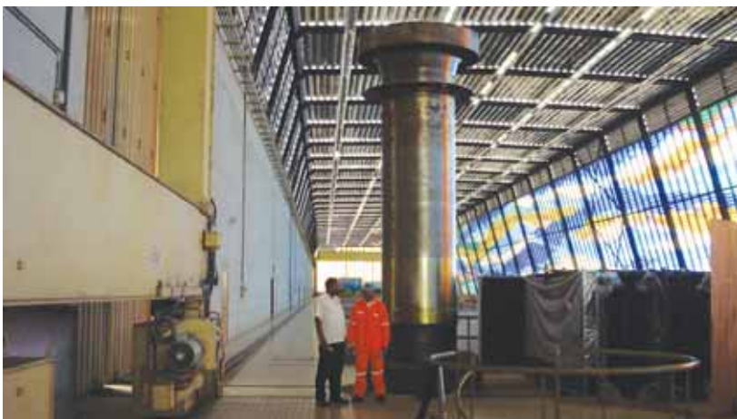
Inga 2: 205 MVA, 56 Pole Rotor & drive shaft
